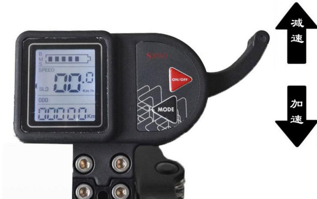
1 Meter contains Acceleration lever ,Start switch button, speed adjustment button and display screen
